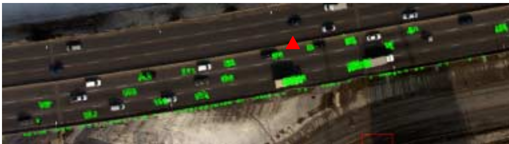
Figure 11. Vehicles extracted from LiDAR data overlaid on the orthoimage.
