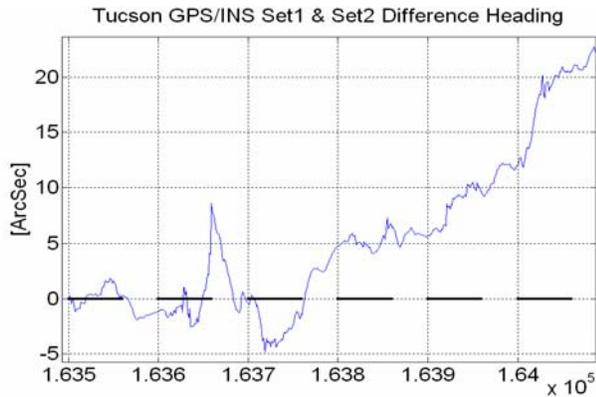
**Figure 5:** The heading difference between the velocity-updated filter and the reference filter over selected time (60 sec) marked with the black lines
