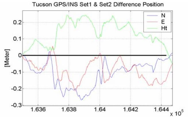
**Figure 7:** The position difference of the velocity update filter
