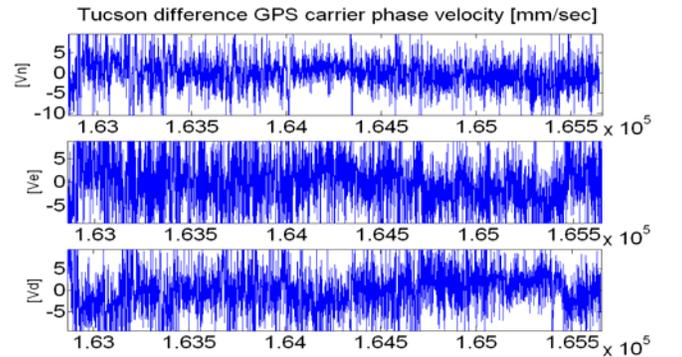
**Figure 2:** The GPS velocity difference in N-E-H between the reference velocity and velocity-based solution
