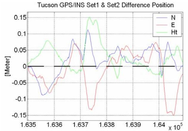
**Figure 3:** The position difference between the velocity-updated filter and the reference filter over selected time (60 sec) marked with the black lines
