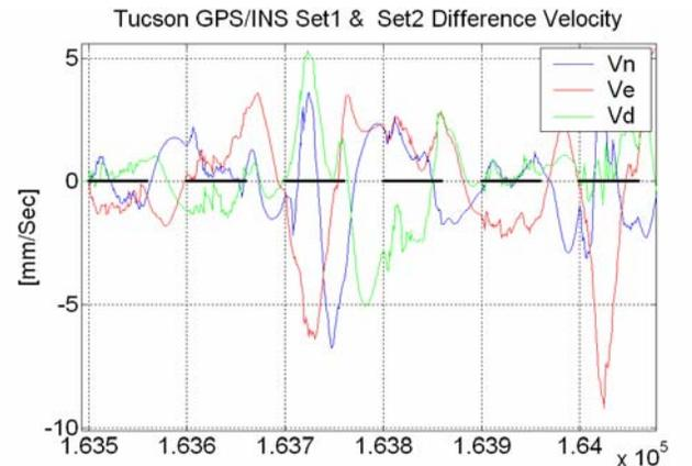
**Figure 4:** The velocity difference between the velocity-updated filter and the reference filter over selected time (60 sec) marked with the black lines
